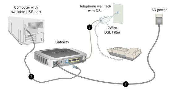
Figure 3. Gateway Connected Via USB
